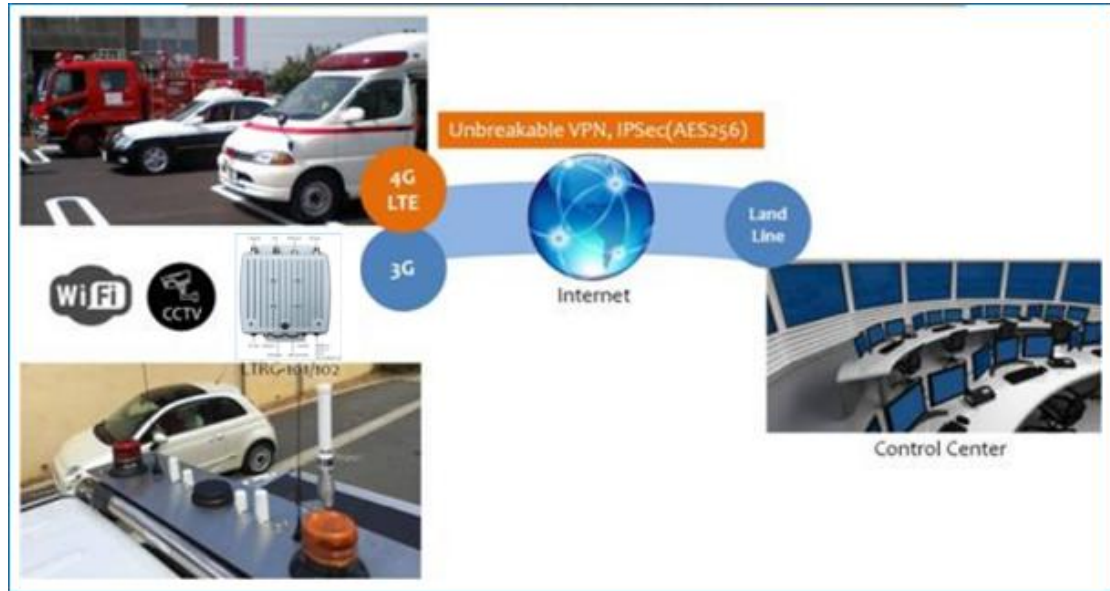
Outdoor 4G modem HYC-OLTRG-101 on vehicle & Control Center
